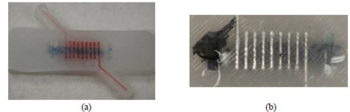
Figure 3. Inductor (a) filled with colored water to verify fluidic isolation and (b) after final fill with liquid metal and ferrofluid
